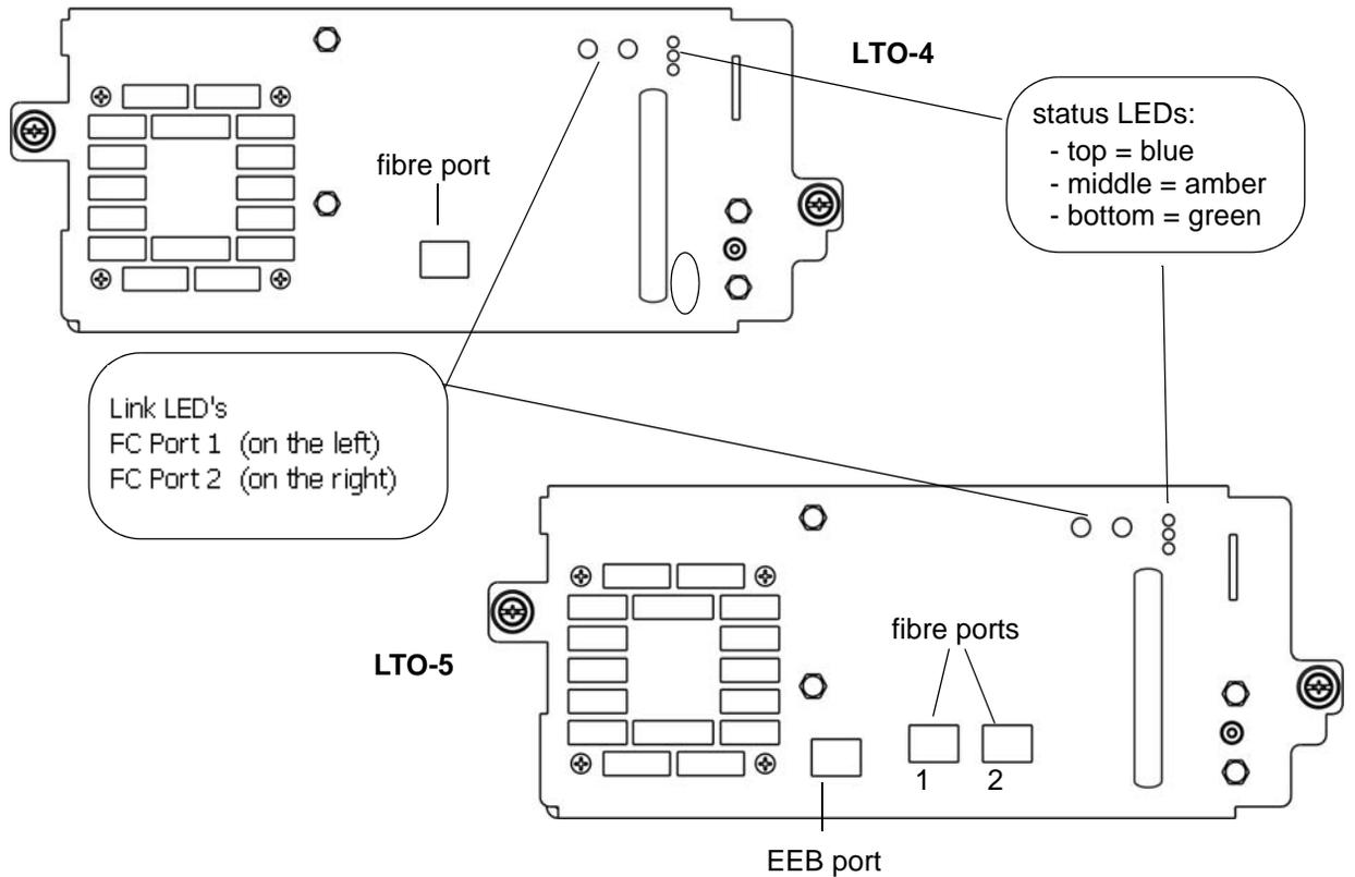
[Table 8](#) on page 92 describes how to interpret the drive sled status LED activity that you might see on the rear of a UDS-2 or UDS-3 drive sled. For a description of how the blade status LEDs appear under normal conditions, see [Table 9](#) on page 92. For information about interpreting the drive link LED, see [Drive Sled Fibre Channel Link LED](#) on page 93.
