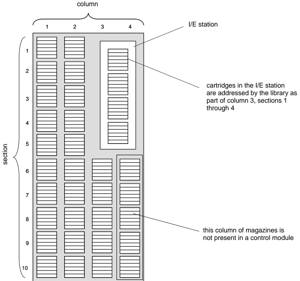
Figure 37 Example - Storage Location Coordinates for Aisle 1, Module 1, and Rack 1
