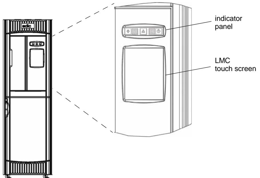
The indicator panel includes a **Robotics Enabled** button with its associated indicator, a **Status** indicator, and a **Power** button with its
