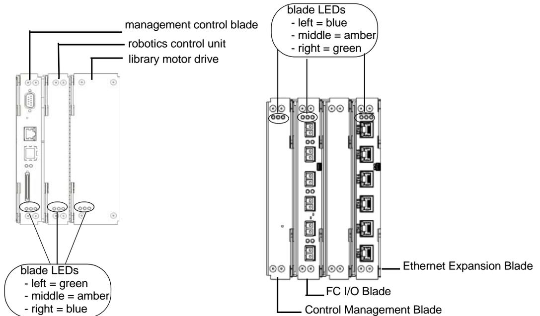
Blade status LEDs provide troubleshooting information that you can use in conjunction with tickets that the library creates. However, the LEDs might not directly correspond to tickets. The LEDs can indicate a firmware or hardware problem so severe that the library cannot create or display a ticket. For example, if the MCB firmware becomes inoperable, the amber LED flashes at 1 Hz, but the library might not be able to display any related tickets.
