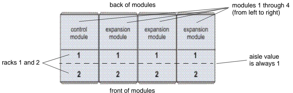
Figure 35 Section, Column, and Row Numbering for Rack 1 - LTO Cartridges
