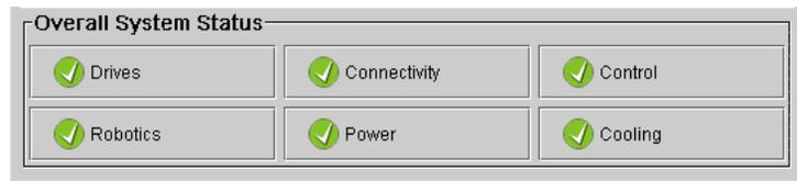
Each button represents a subsystem. [Table 37](#) shows the library subsystems and some of the components that each subsystem represents. Each field replaceable unit (FRU) in the library belongs to one of the subsystems.
