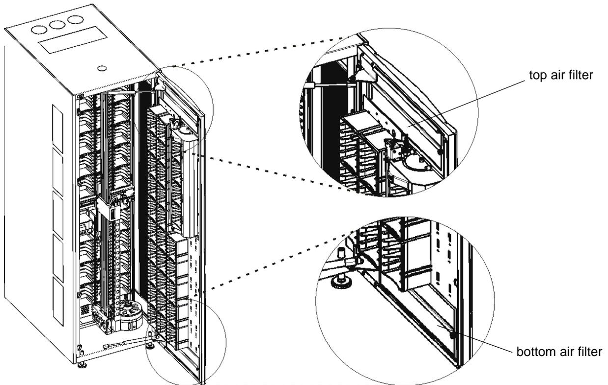
Many factors exist that contribute to the need to regularly service the air filters. For example, the total number of tape drives and the operating environment greatly affect the rate at which debris accumulates in the air filters.
