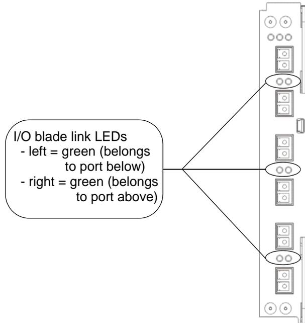
[Table 12](#) on page 96 describes how to interpret the link LED activity that you might see. There are two different models of FC I/O blade: 6404 and 7404. LED behavior varies based on which model is installed in the library.
